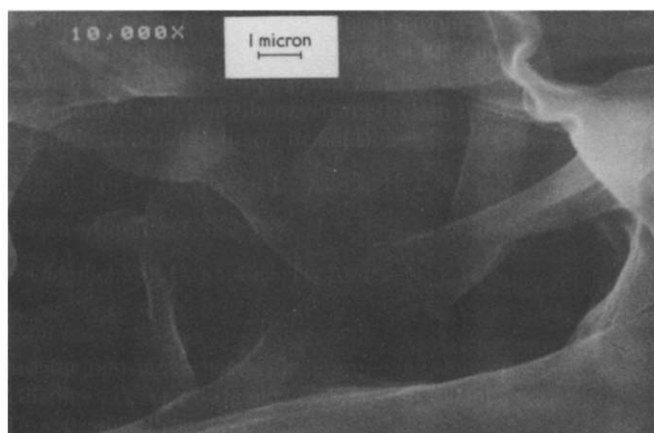
Figure 1 Scanning electron micrograph of the network structure of a 'fuzzy sphere' polyelectrolyte complex
